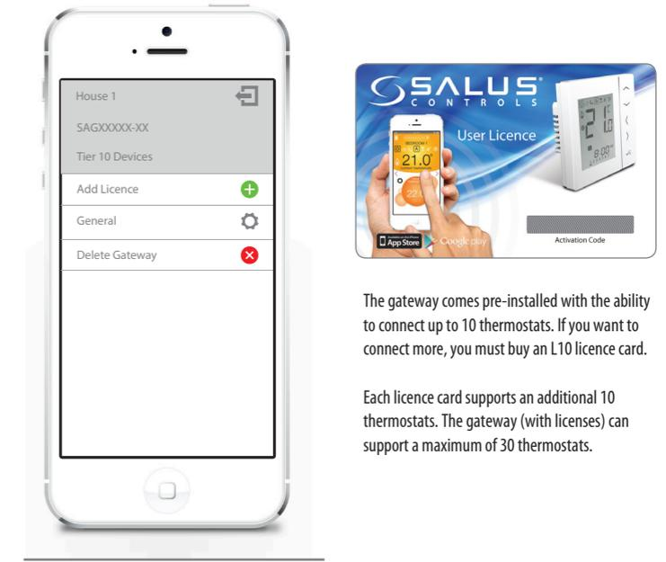
The gateway comes pre-installed with the ability to connect up to 10 thermostats. If you want to connect more, you must buy an L10 licence card.
